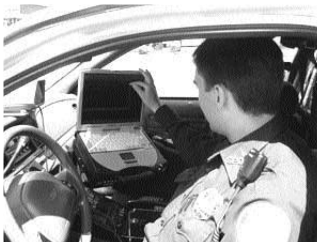
The laptop computer is mounted on the dashboard next to the driver for easy access.
